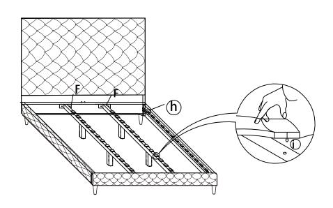
STEP 7 Insert small slat (I) into plastic slats (h, i) as shown in diagram. Attach long slat (L) to Siderail (E) with bolt f as shown.
