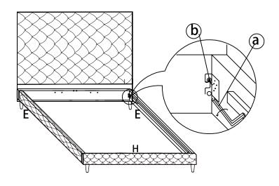
STEP 4 Attach center support (F) to headboard (G) by using bolt (b) through washers (e, d) as shown in diagram.
