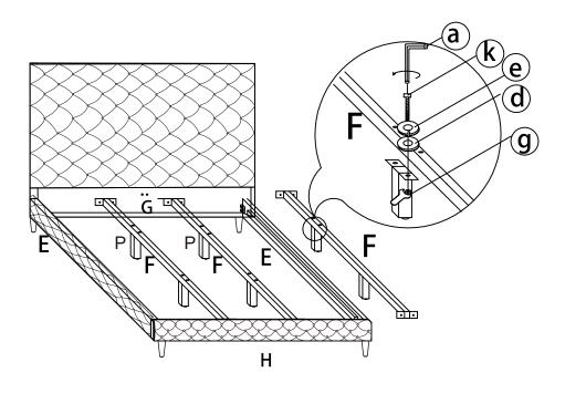
STEP 6 Insert center plastic slot ( i ) into holes on center support bar (F). Press firmly into place as shown in diagram. Attach rail plastic slat ( h ) using same procedure.
