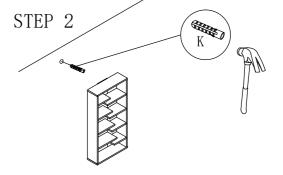
1. Use a light hammer to tap anchor into hole. 2. Anchor should fit snugly. If hole is too small, drill again to increase hole size . Do not force anchor into wall.
