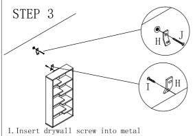
bracket and into drywall anchor.
