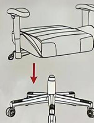
5 Align ①&⑪ with the holes of seat, then tighten screws.
