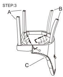
Use the enclosed hardware pack for leg assembly, "IMPORTANT" Donot fully tighten bolt on this step, only tighten "HALF WAY".
