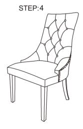
Turn around the chair seat on floor to make sure four legs are aligned and fully tighten all bolts from previous step with allen key.
