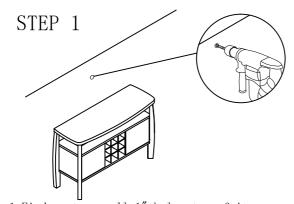
1. Find spot on wall 1" below top of item. 2. Using a drill bit slightly thinner than anchor, drill hole into drywall.
