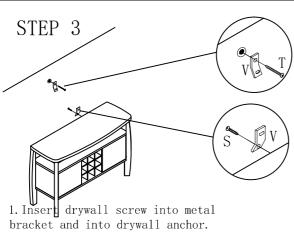
2. Insert flathead screw into second metal bracket and into back of item along top edge.
