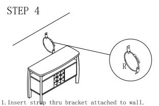
1. Insert strup thru bracket attached to wall. then thru bracket on item, and into head of strap. 2. pull lightly til strap stops.
